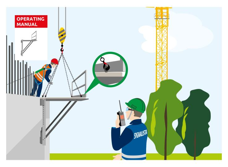
Transport and installation of clamps for platforms should be done in accordance with ISPW for carpentry and reinforce concrete works, and with an operating manual or a design for formworks.
