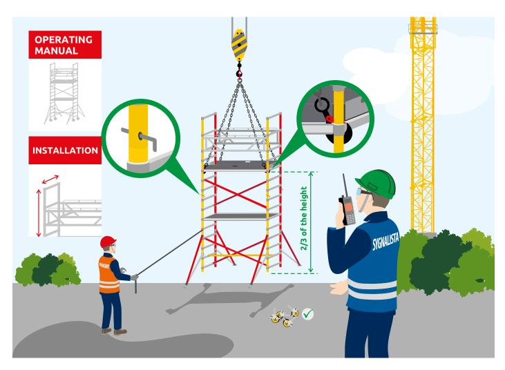
The scaffolding should be transported in accordance with the manufacturer's operating manual. When the manual does not provide information on a method of transporting the scaffolding, an individual design for its lifting should be prepared, taking into account the guidelines below.
