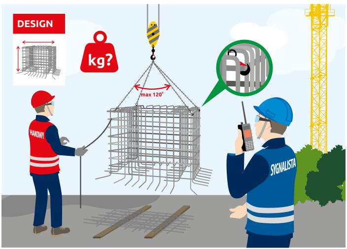
Conduct transport in accordance with the reinforcement design or designer's guidelines, specifying sling attachment points.
