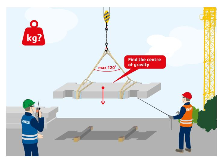
For the transport of road slabs without lugs use two choker belt slings wrapped twice around the load, fastened at 1/4 of their length from the edges, and attached to a chain sling.
