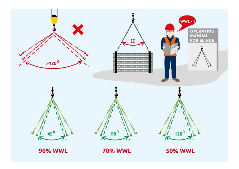
The working load limit for double- and multi-leg slings depends on a top angle value measured at a diagonal between legs, and amounts to:
