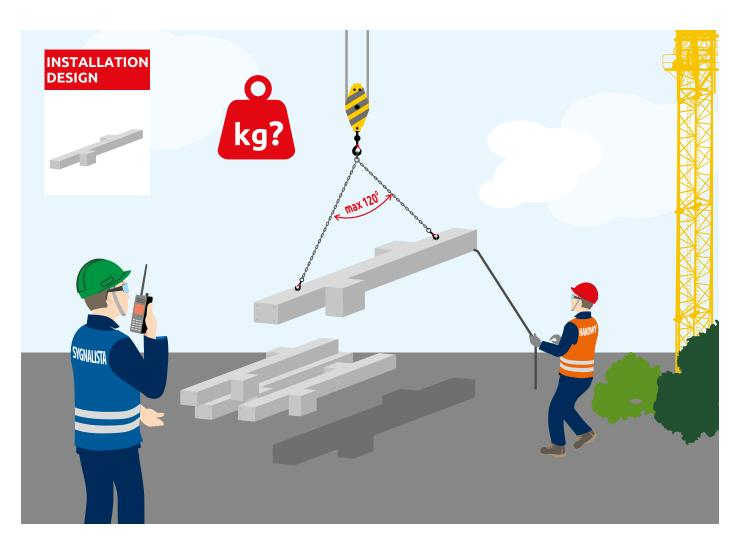
Conduct transport in accordance with the installation design or guidelines of a component manufacturer. During the transport of prefabricated reinforced concrete piles, ensure that:
