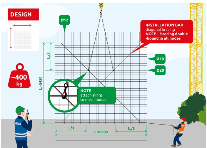
Conduct transport in accordance with the design or designer's guidelines, specifying a way for attaching the mesh.
