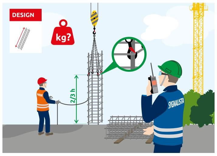
Conduct transport in accordance with the design or designer's guidelines, specifying points for attaching the element.
