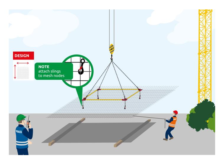
• Alternately, use a beam. Attach a flooring mesh to the beam at its bottom bars.
