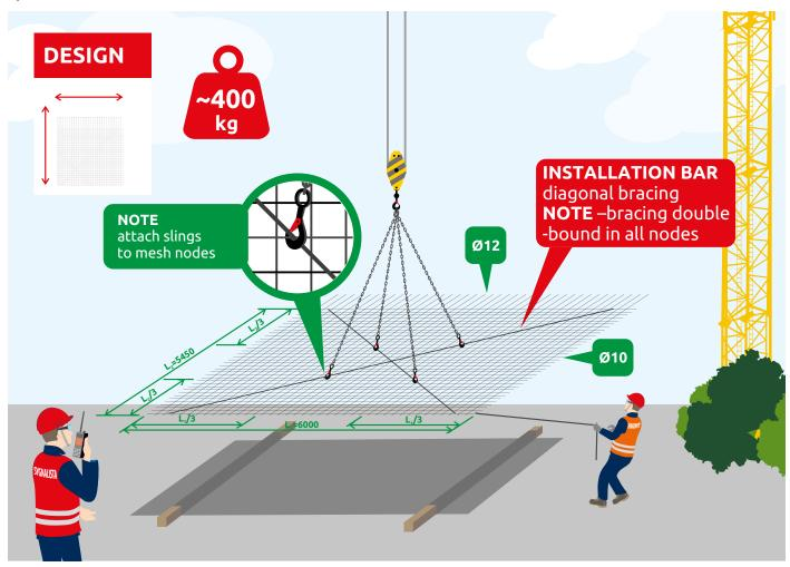
Conduct transport in accordance with the design or designer's guidelines, specifying points for attaching the mesh.
