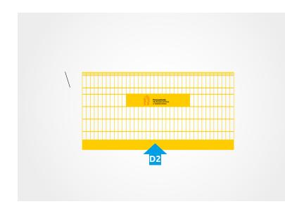
A safety mesh is used to protect against fall from height of people and tools and must meet the requirements of PN-EN 13374. Mesh used on the edge must have a tight toeboard (at least 15 cm).
