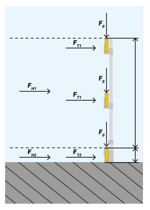
Key **F**<sub>o</sub> - 1,25 kN **F**<sub>11</sub> - 0,3 kN (maximum deformation of 55 mm)
