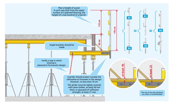
Requirements concerning operational load of a working platform must result from a manufacturer's instruction or an individual design.
