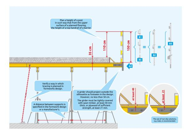
Requirements concerning operational load of a working platform must result from a manufacturer's instruction or an individual design.
