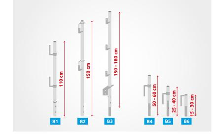
Use a post of appropriate height, so a top handrail of the barrier meets the minimum height, taking into account the flooring thickness or the peripheral beam height.
